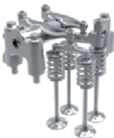
Blow down Driven by exhaust back pressure
